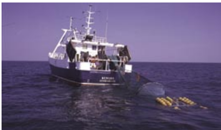
FIGURE 11 Setting out the trawl, codend cover and collection cage-unit from a trawler. The cover around the codend is supported by two hoops. The timers of the release-unit can be seen on the surface.
