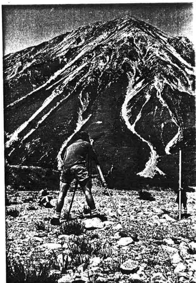
Fig. 8b: A 3 man party using a surveyor's level and staff to measure a stream-bed profile. Peveril Peak (Poulter Catchment) in background.
