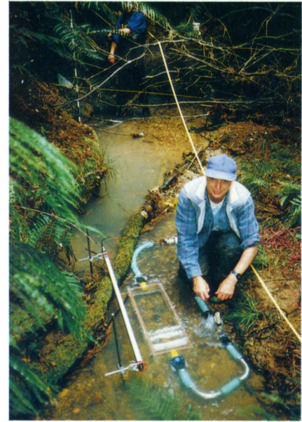
Above: Part of an environmental study looking at the effects of forestry on streams. NIWA staff measure benthic metabolism and current velocity
