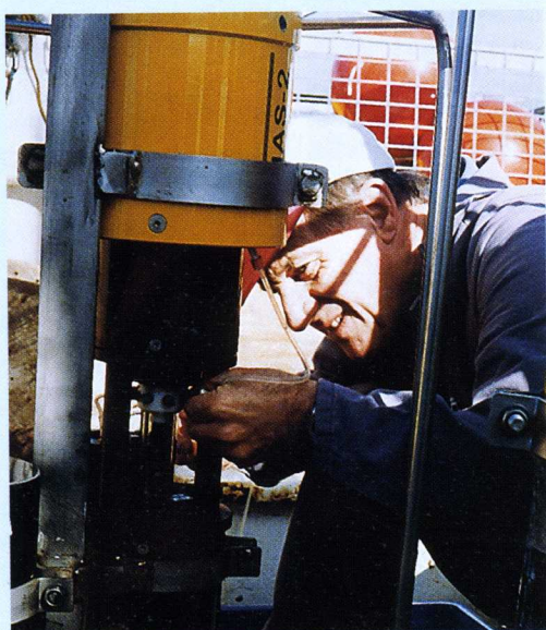
Figure 4 Stuart Pickmere (NIWA, Hamilton) services the in situ nitrate analyser during one of the 1996–97 voyages. A battery pack in the lower compartment powers a multiport syringe (centre), which mixes reagents from the upper compartment with a seawater sample. This is assayed photometrically, following cadmium reduction and colour development, and the data are stored.
