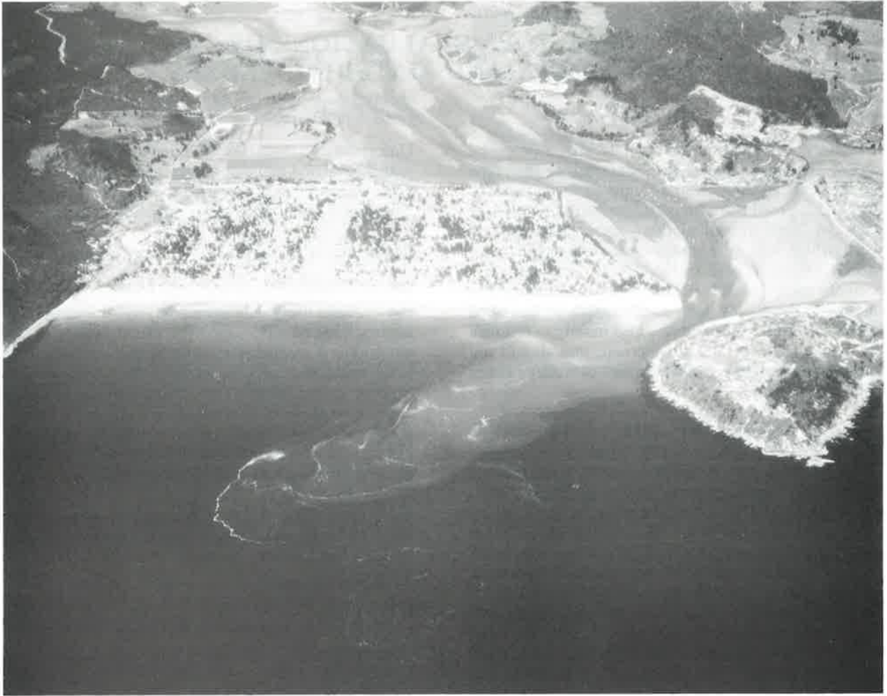
Figure 2.11 Tairua Estuary entrance, showing the ebb tidal jet exiting the entrance and the resulting suspended sediment plume. Changes in longshore current, imprinted on the plume shape, have occurred early in the ebb tide phase, but generally the current to the left will ensure predominantly 'new' water will enter the estuary from the right. Photo taken by Whites Aviation in 1984.
