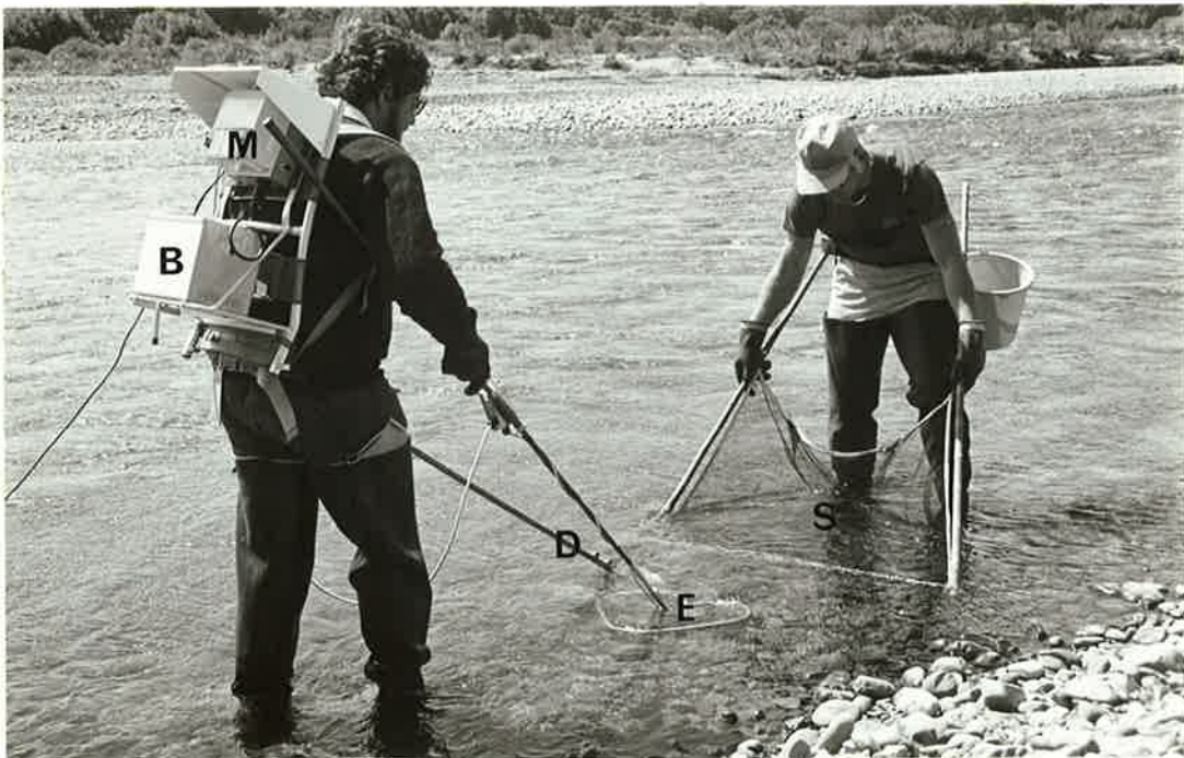
FIGURE 3b. Pack-set electric fishing system: essentially the same as generator powered fishing, except the power source, a lead-acid battery (B), and the electric fishing machine (M) are carried on the operator's back - thus no cable reel is necessary. In both systems, fish stunned by the electrode (E) either drift downstream into the stop-net (S) or are collected in the operator's dip net (D).
