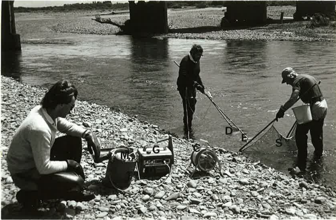
FIGURE 3a. Generator powered electric fishing system: power is provided by a 230-volt a.c. generator (G). The electric fishing machine (M) converts the electricity to pulsed d.c., which is supplied to the operator's electrodes (E) through the cable (C). Note the use of rubber gloves and waders by the operator and assistants, and the bucket for holding the catch.
